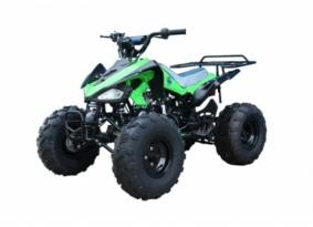
A Throttle Regulator provides total control over the Versatile 125cc 4-stroke Air-cooled Engine by limiting speed to as low as 10 mph, or all the way up to 35 mph and anywhere in between, your choice!. A Starter/Brake Interlock prevents accidental starting, and a Lanyard Safety Cutoff will shutdown the engine if separated from the quad.
