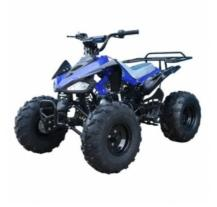
A Throttle Regulator provides total control over the Versatile 125cc 4-stroke Air-cooled Engine by limiting speed to as low as 10 mph, or all the way up to 35 mph and anywhere in between, your choice!. A Starter/Brake Interlock prevents accidental starting, and a Lanyard Safety Cutoff will shutdown the engine if separated from the quad.
